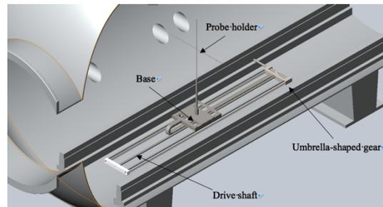
Figure 1. Rail and moving component systems inside the vacuum chamber.
