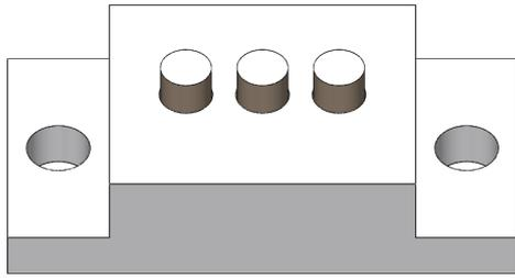
Figure 2 Overall layout of 3D probe array.
