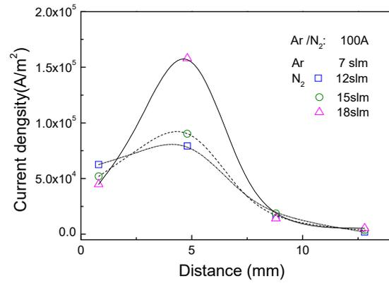
Fig. 3 Current density distributions along the axial distance of the generator (0: the anode throat exit).
