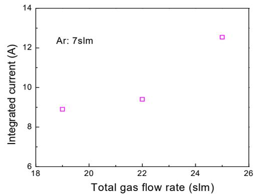
Fig. 4 Variations of the integrated arc current as total gas flow rate.
