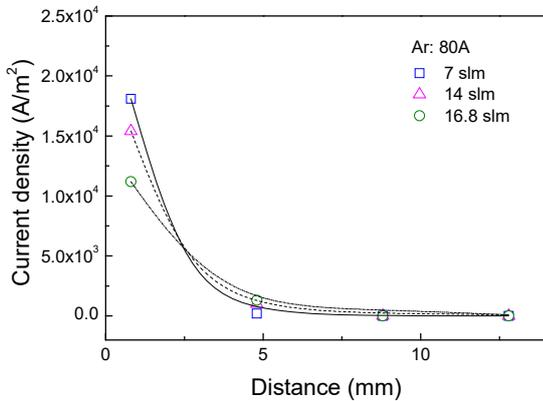
Fig. 2 Current density distributions along the axial distance of the generator (0: the anode throat exit).
