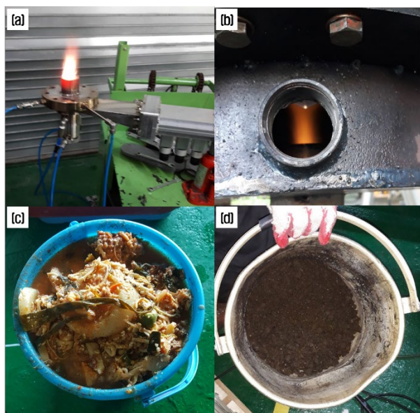
Fig. 2. Photograph images of LPG plasma burner flame at (a) 2 kW power and (b) in the reactor, and (c) before and (d) after food waste of torrefaction.
