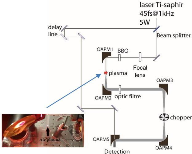
Fig. 1. Experimental setup based on two-colours air-breakdown terahertz generation. Off-axis parabolic mirrors (OAPM) are used for beam (optical and THz) shaping.
