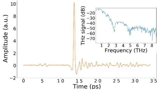
Fig. 2. Terahertz waveform generated by the experimental setup (schematised in Fig. 1), and coherently detected using electro-optic detection, and its associated intensity spectrum (inset).
