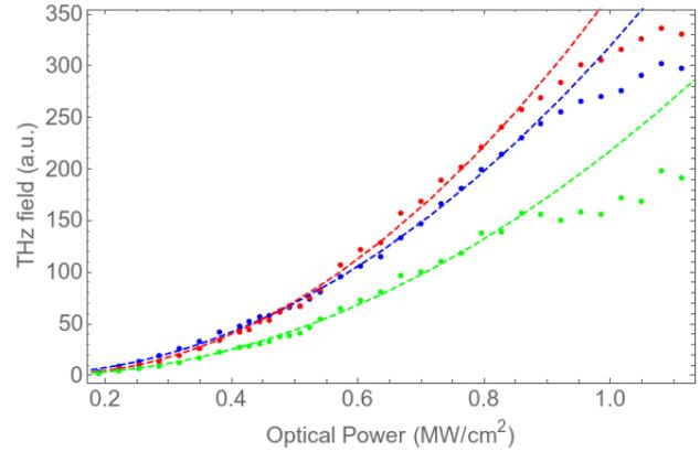
Fig. 3: THz E-field generated by two-colours air breakdown process in air (blue dots), in nitrogen (red dots), and in helium (green dots) versus the optical fluence at the focal point, and their associated quadratic fitting curves (dashed lines).
