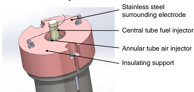
Fig. 1. Description of the Gliding arc plasma system implementation on the burner
