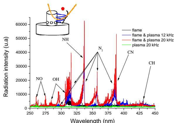
Fig. 5. Effect of the plasma within the flame at the edge of the electrode.  $Q_{TOTAL} = 169$  L/min,  $\phi = 1.2$ , Swirl 1.4
