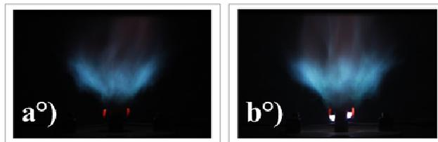
Fig. 2. Photo of the turbulent flame with swirler ( $Sn=1.4$ ): a°) without GAP and b°) with GAP.  $Q_{AIR} = 150$  L/min,  $Q_{CH4} = 19$  L/min and  $P_{FLAME} = 11.3$  kW.
