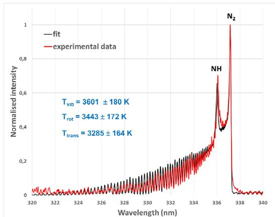
Fig. 6. Example of fit on the 320 -340 nm emission spectrum in plasma assisted combustion.  $Q_{TOTAL} = 169$  L/min,  $\phi = 1.2$ , Swirl 1.4,  $f_{PLASMA} = 20$  kHz
