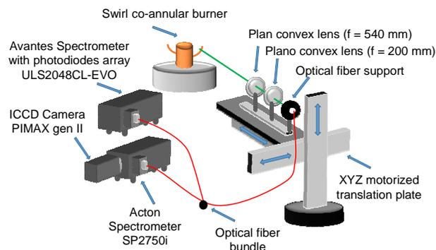
Fig. 3. Schematic view of the optical setup for OES experiments
