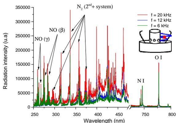
Fig. 4. Effect of the pulse frequency on the plasma radiation:  $Q_{AIR} = 30$  L/min,  $U_{ARC} = 230$  V
