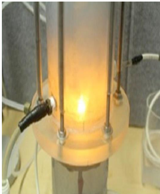
Fig.1 Gliding Arc Plasmatron Submerged into Liquid Solution
