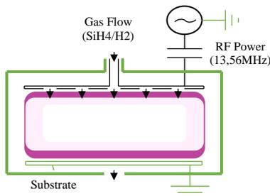
Fig.1. Schematic representation of the axis symmetric radio-frequency reactor.
