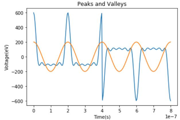
Fig.2. Peaks and Valleys waveforms for different harmonics. The blue curve corresponds to  $N_{RF}=5$ , the orange curve corresponds to  $N_{RF}=1$ . [5].
