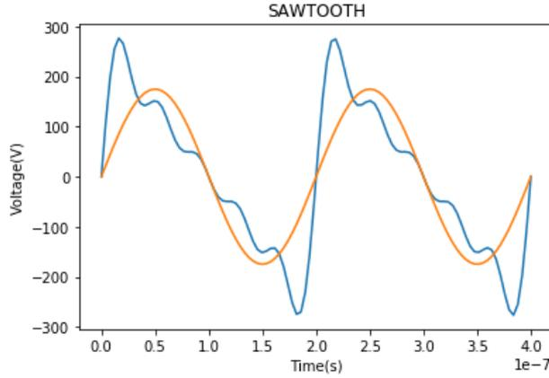
Fig.3. Sawtooth-like waveforms. Sine (orange line) and refined (blue line) waveform across two periods. The number of harmonics for the sawtooth-like waveform (blue curve) is  $n = 5$  [6].
