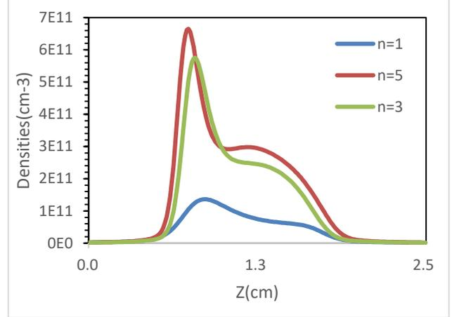
Fig.5. Time-averaged density of  $\text{SiH}_3^+$  along the axis of symmetry of reactor for different numbers of harmonics, namely  $n=1, 3, 5$ .
