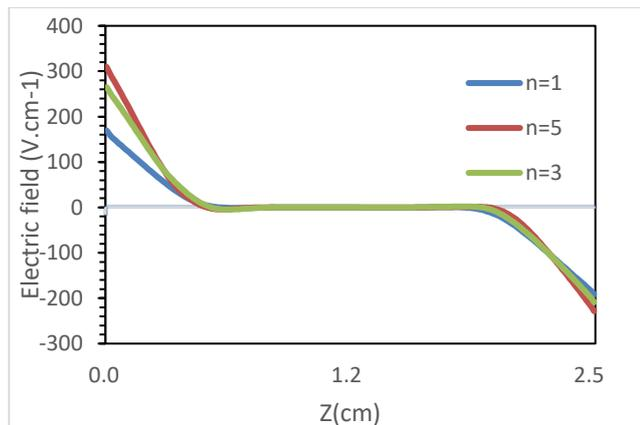
Fig.4. Time-averaged electric field along the axis of symmetry of reactor for different numbers of harmonics, namely  $n=1, 3, 5$ .
