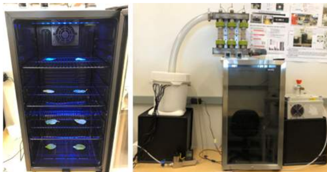
Fig. 1. On the left, spinach leaves are inside the refrigerator, where treatment occurs. On the right is an overall view of the system.
