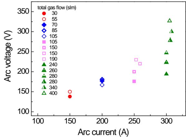
Fig.3 Arc voltage changed as the change of total nitrogen flow rate at different arc current.
