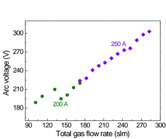
Fig.4 Arc voltage changed with the total gas flow rate of nitrogen at 200 A and 250 A.
