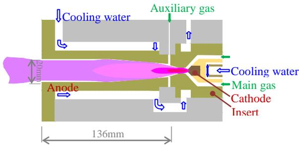
Fig.1 Schematic drawing of the generator structure and working situations.
