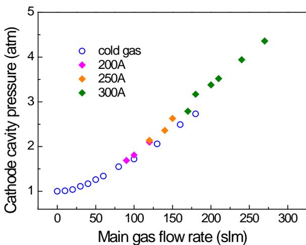
Fig.2 Pressure in the cathode cavity changed as the main gas flow rate of nitrogen at different arc current for plasma igniting.
