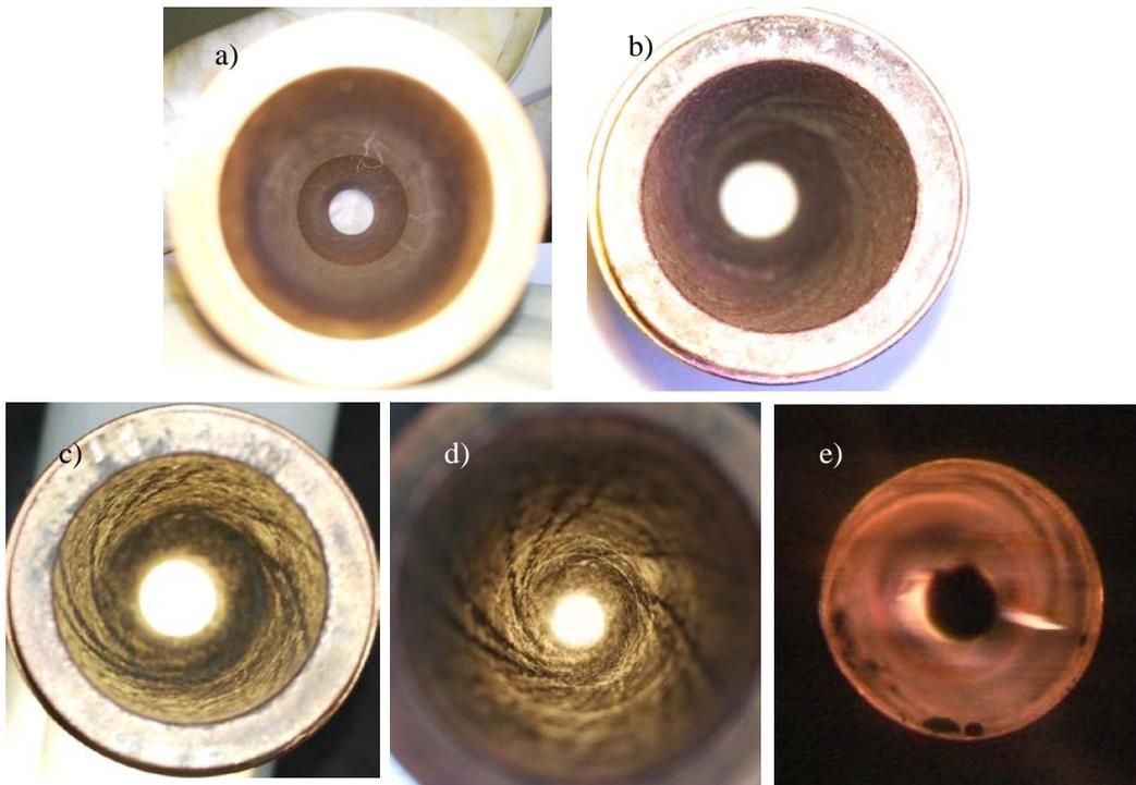
Fig.6 Pictures of the anode channel surface after the ignition, a)  $N_2$ -main/Ar-auxiliary gas, b)  $N_2/N_2$  gas, c)-d) air/air gas. e) during the ignition of air/air with the copper mirror reflecting and camera exposure time of 250  $\mu s$  through a filter of 1% transmittance.
