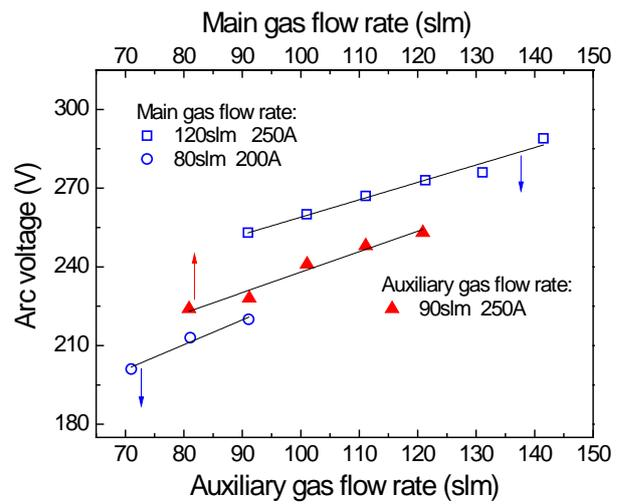
Fig.5 Arc voltage changed with the main or auxiliary gas flow rate of air at set another gas flow rate and arc current.
