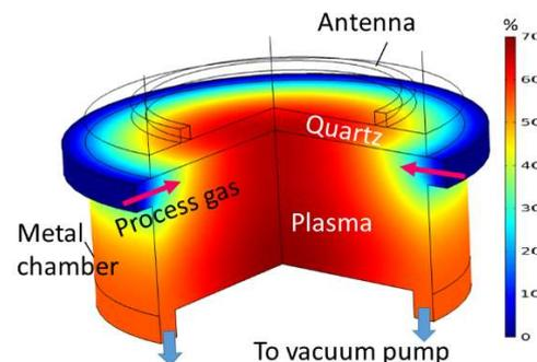
Fig. 1. Degree of dissociation of chlorine in high-density low-temperature low-pressure ICP.
