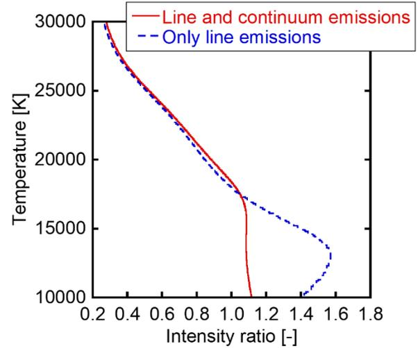
Fig. 2. Relationship between relative intensity and temperature for BPFs combination of  $480\pm 5$  nm and  $500\pm 5$  nm in 50vol%N<sub>2</sub>-Ar.
