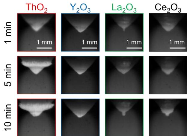
Fig. 4. Image of cathode measured at 785 nm wavelength at 1, 5 and 10 min after ignition.
