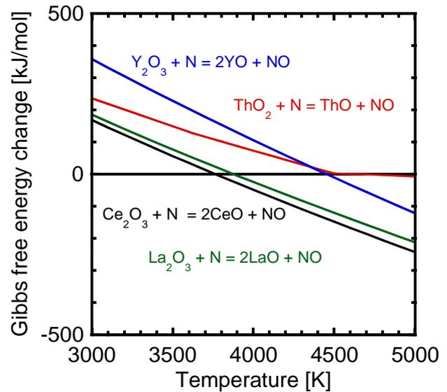
Fig. 7. Gibbs free energy for the reaction of a nitrogen radical with a metal oxide.
