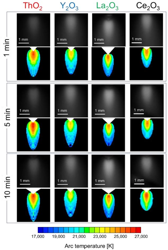
Fig. 5. High-speed snapshots of arc and corresponding arc temperature distributions at 1, 5, 10 min after ignition.
