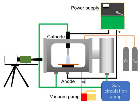
Fig. 3. Schematic diagram of DC arc system.
