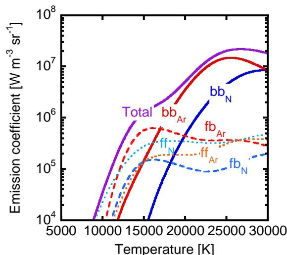
Fig. 1. Temperature dependence of emission coefficients in 50vol%N<sub>2</sub>-Ar arc with the BPF of 480±5 nm. bb: line emission, fb: recombination radiation, ff: bremsstrahlung emission.
