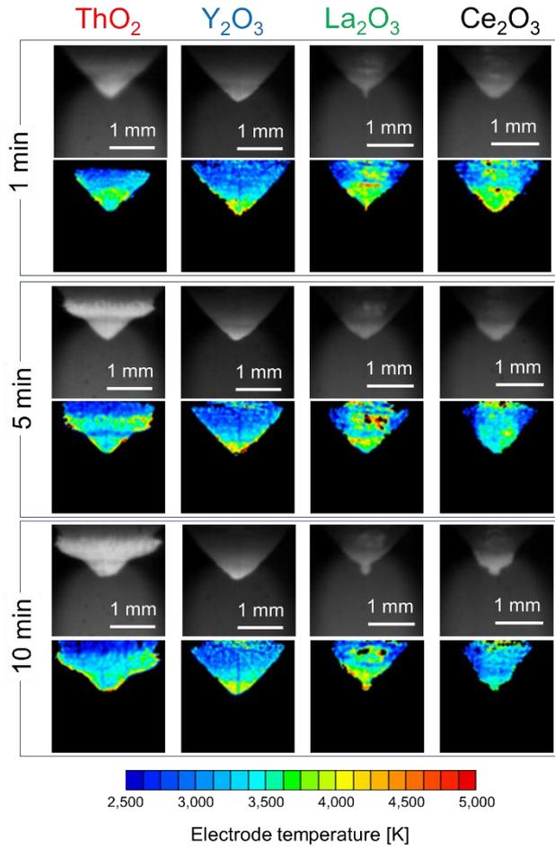
Fig. 6. High-speed snapshots of electrode and corresponding electrode temperature distributions at 1, 5, 10 min after ignition.
