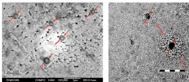
Fig.1 SEM and TEM pictures of Carbon-Carbon nanocomposite thin films formed in  $C_2H_2$ ,  $P=800$  W,  $p=0.1$  Pa.
