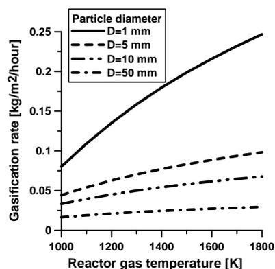
Fig. 1. Dependence of rate of gasification of wooden particles on temperature of gas in reactor
