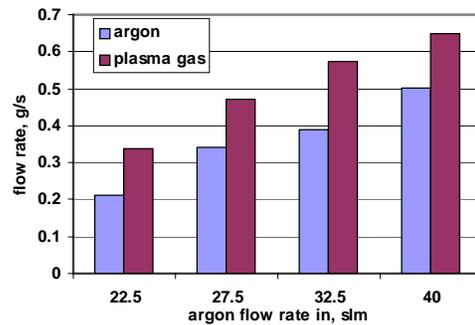
Fig.3 Effect of supplied argon flow rate on argon flow in generated plasma jet and on total plasma gas flow rate for  $I=500$  A.
