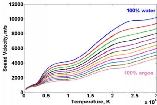
Fig. 5 Sound velocity as a function of temperature and plasma gas composition.
