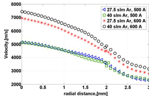
Fig. 6 Velocity profiles in plasma flow for different plasma torch operation parameters.
