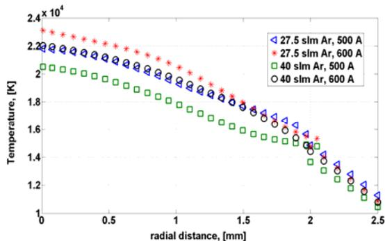
Fig.2 Temperature profiles in plasma flow for different plasma torch operation parameters.
