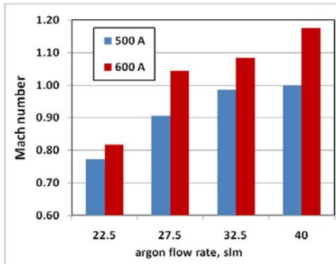
Fig. 4 Mach number at the torch exit as a function of secondary gas flow rate for two arc currents.
