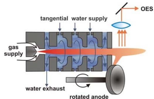
Fig.1 Hybrid gas-water torch and applied diagnostics.
