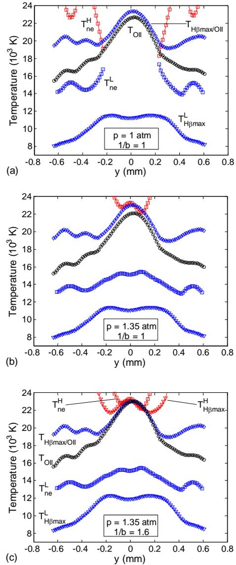
Fig. 2 Radial temperature profiles at the nozzle exit obtained from electron number density and absolute and relative emission coefficients of  $H_\beta$  and O II for the pressure (a) 1 atm, (b) 1.35 atm, and (c) 1.35 atm and absolute emission coefficients multiplied by a factor of 1.6.
