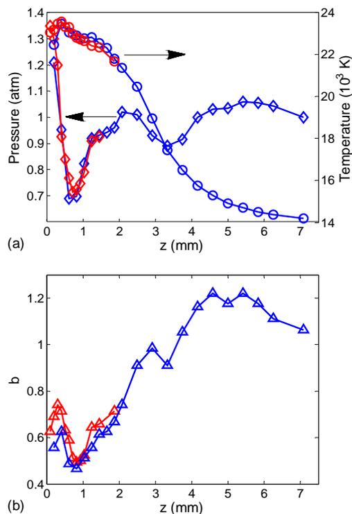
Fig. 4 Axial profiles of (a) the pressure and temperature and (b) the effective population factor.
