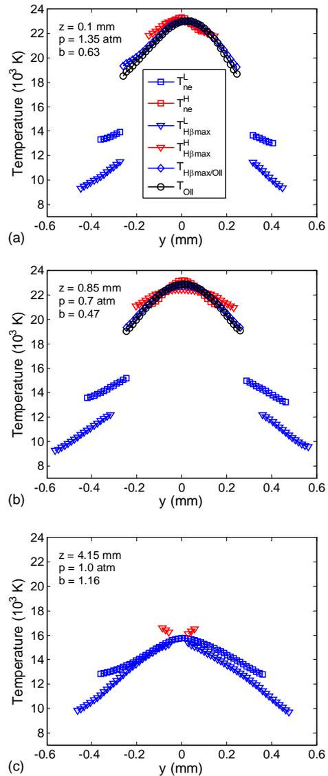
Fig. 3 Radial temperature profiles at three distances  $z$  from the nozzle exit.
