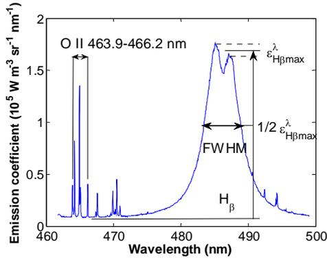
Fig. 1 Emission spectrum with  $H_\beta$  and O II lines.
